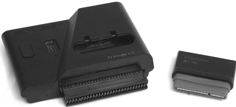
Fig 1.13 The ZX Interface 2 with a ROM cartridge. The interface also doubled as a joystick interface for the Sinclair joystick standard.
